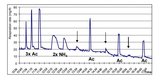
Respiration experiment with mixed textile wastewater. arrows indicate additions of 50 ml of wastewater. Ac = addition of acetate. NH4 = addition of ammonium.
