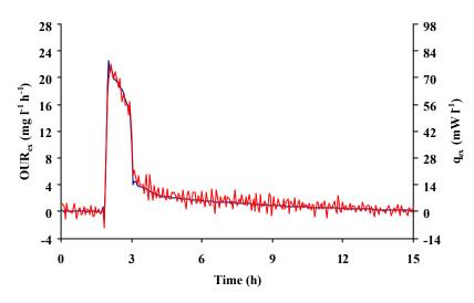
Comparison between OUR (smooth line) and heat production rate (noisy line) profiles simultaneously acquired (raw wastewater B. AS plant biomass).
