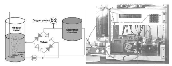
Schematic representation and photo of the used respirometer
