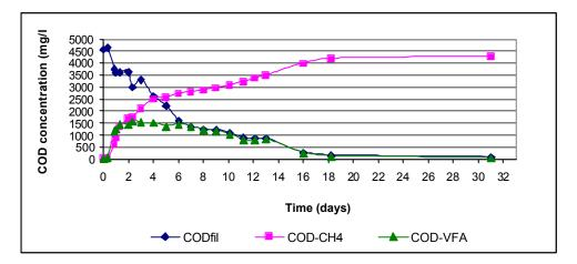
Anaerobic biodegradation of sizing wastewater. measured as COD concentrations.
