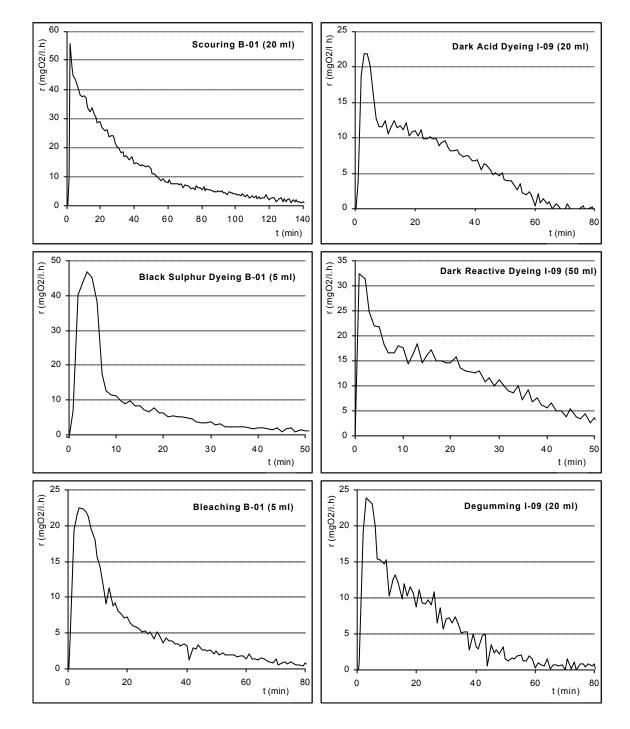
Single respirograms like these have been selected and will be used for parameter estimation. An activated sludge model for textile wastewater characterisation based on respirograms was developed and implemented in Matlab. In cooperation with Partner 6 (EI/JRC) a comparison was made between respirometric and calorimetric experimental results with the same wastewater-sludge combination (WP05.03.6).
